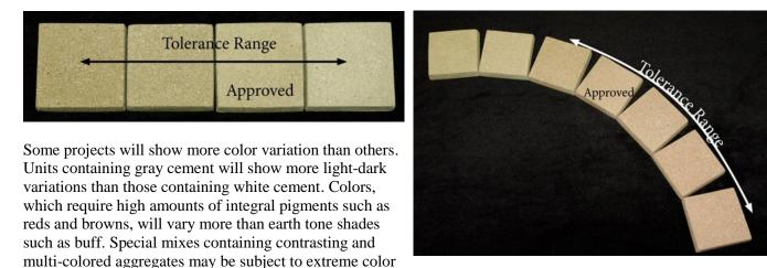
Variations in color within the same stone may be caused by efflorescence or free lime migrating to the outer surface. This can usually be remedied by proper cleaning. Staining, mortar smears or uneven washing can also cause color variations. These variations are not necessarily inherent in the cast stone but as a result of installation or post construction cleaning. In such instances, the manufacturer should be consulted for recommended treatment of these variations.
