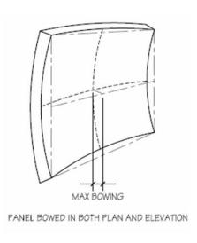
A problem encountered in the field is that convex bowing cannot be measured as shown after the stone has been
